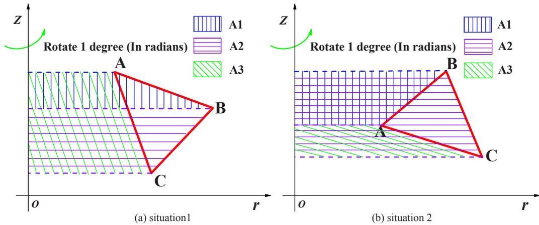
Fig. 3. Combination and split method to determine the control volume
