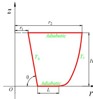
Fig. 5. Computational domain and boundary conditions
