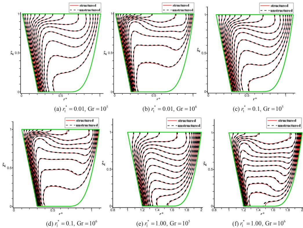
Fig. 7. Comparison of temperature fields with different computation parameters
