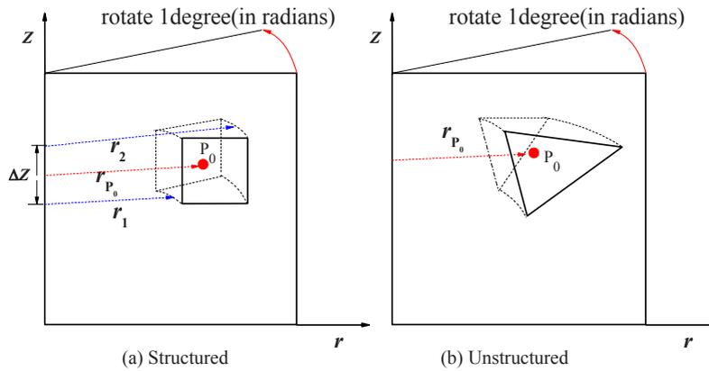
Fig. 1. Sketch map of structured and unstructured control volumes in a two-dimensional cylindrical coordinate system
