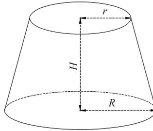
Fig. 2 Circular truncated cone formed by rotating a right trapezoid by 360 degrees
